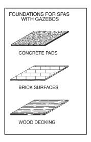
If you are purchasing a deck package or a spa enclosure with your spa, a solid foundation becomes mandatory. Placing them on any surface other than a single level pad could create problems with their installation. Pictured at right are a few of the recommended surfaces.
