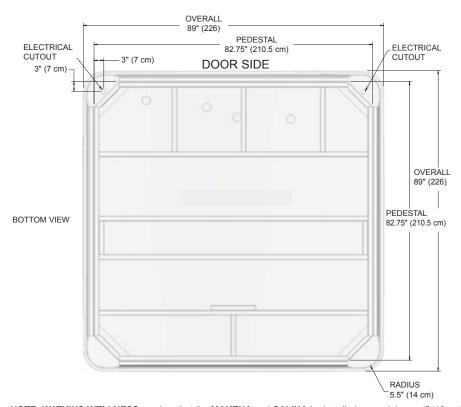
**NOTE: WATKINS WELLNESS** requires that the **MAKENA** and **SALINA** be installed on a minimum 4" (10 cm) thick reinforced concrete pad or structurally sound deck able to support the "dead weight" found in the chart on the back page.
