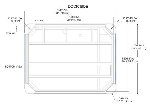
**NOTE: WATKINS WELLNESS** recommends that the **KAUAI** be installed on a minimum 4" (10 cm) thick reinforced concrete pad or structurally sound deck able to support the "dead weight" found in the chart on the back page. **WARNING:** The **KAUAI** must not be shimmed in any manner.
