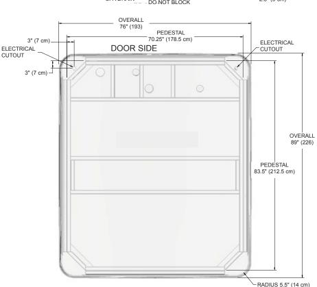
**NOTE: WATKINS WELLNESS** recommends that the **MARTINIQUE** be installed on a minimum 4" (10 cm) thick reinforced concrete pad or structurally sound deck able to support the "dead weight" found in chart on the back page. **WARNING:** The **MARTINIQUE** must not be shimmed in any manner.
