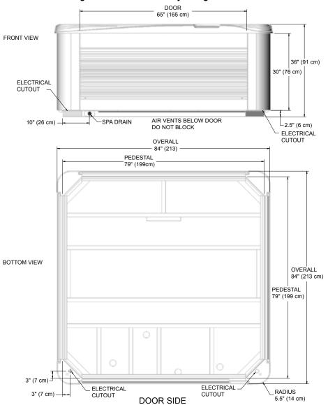
**NOTE: WATKINS WELLNESS** recommends that the **SEYCHELLES** be installed on a minimum 4" (10 cm) thick reinforced concrete pad or structurally sound deck able to support the "dead weight" found in the chart on the back page.
