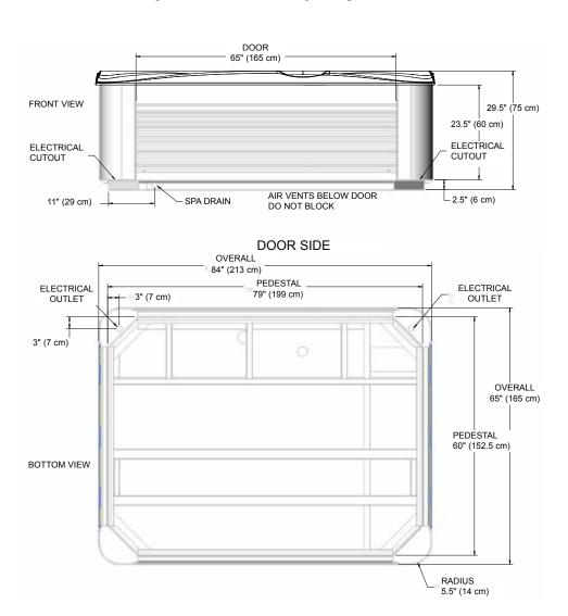
**NOTE: WATKINS WELLNESS** recommends that the **KAUAI** be installed on a minimum 4" (10 cm) thick reinforced concrete pad or structurally sound deck able to support the "dead weight" found in the chart on the back page. **WARNING:** The **KAUAI** must not be shimmed in any manner.
