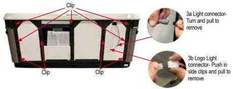
Pull bottom door panel away (using both hands spaced shoulder length apart) from each side of the spa center, this may require a slight amount of force because of the upper clips until they all un-clip. Lower panel to ground. Disconnect both the logo light and front light wires from door panel, then remove door panel from spa area and set in a cool shaded place. Remove foam to access.
