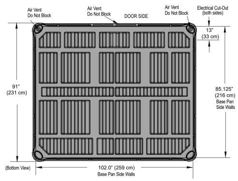
NOTE: **WATKINS WELLNESS** requires that the **CANTABRIA** be installed on a minimum 4" (10 cm) thick reinforced concrete pad or structurally sound deck able to support the "dead weight" found in the spa specification chart.
